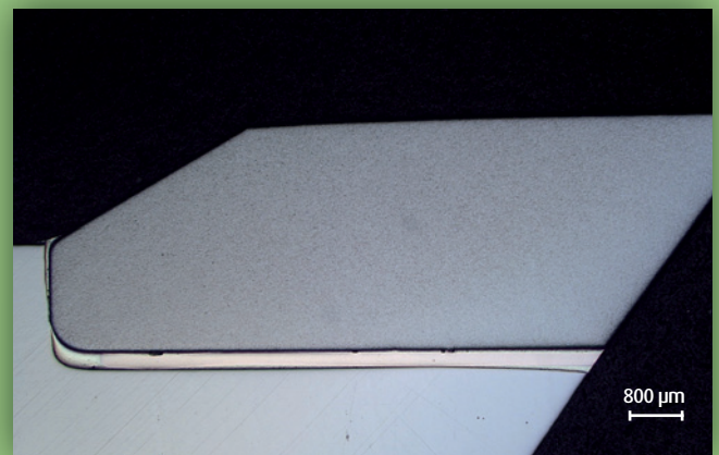
Figure 29 | Cemented carbide saw tooth brazed using BrazeTec 49/Cu but directly in contact with the steel substrate [38]
