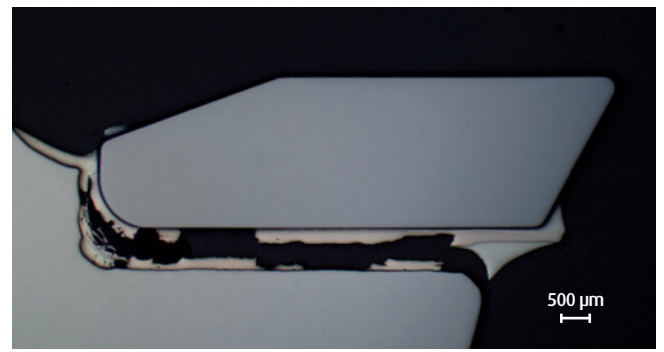
Figure 27 | Cemented carbide saw tooth brazed using BrazeTec 49/Cu showing a failed joint in the copper interlayer [37]
